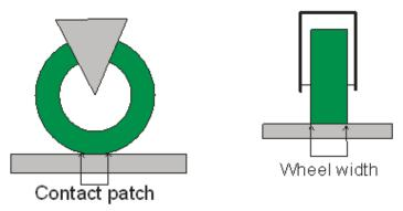
This is shown in the next schematic, where the contact patch is effectively calculated as a rectangle, in the method used above.
