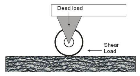
A typical example of a dynamic load is shown in the following diagram, a roller trolley or pallet jack wheel on a floor. For the purposes of this discussion, we restricted the discussion to dead loads, since shear and dynamic loads are hard to quantify, and the involved forces are more complex to analyse.
