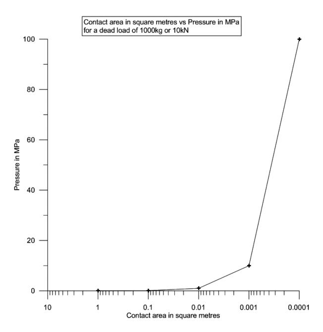
This can be seen in the following graph where a 10kN force (1000kg or 1 tonne dead load) is applied to a floor with differing contact areas for the force/load to be applied over
