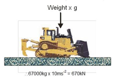
The force exerted by the load of the bulldozer is then supported over the area of its caterpillar tracks on the ground to indicate how much pressure it creates on the ground surface (called ground pressure).
