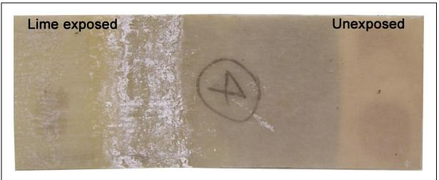
Figure 1. An example of a polyester resin shower base exposed to alkaline water for three months. A degree of corrosion is visible on the left of the sample and is visible as the white deposits.
