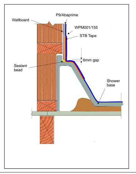
Figure 4. An example of a wall tray detail where fibre-cement sheets are placed onto a preformed shower base. Note STB tape over the sealant filled joint.
