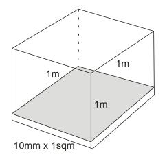
From these figures, it is then possible to determine whether the tile is a suitable weight for the substrate, and/or whether it requires the use of mechanical supports for heights above 3m.
