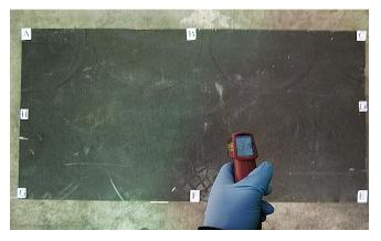
Conducting a sun exposure trial of a large format 'blue stone tile'. Measuring the surface temperature of the tile. The letters mark the positions for measurement with a straight edge laid across the tile. This measures the unrestrained movement of the tile.
