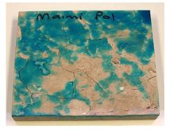
An example of a stone tile with significant potential for moisture marking
