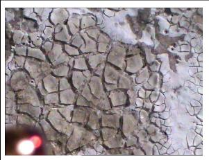
Photomicrograph of primer that has been decomposed by alkali hydrolysis as a result of contact with the damp treated concrete shown in the picture on the left
