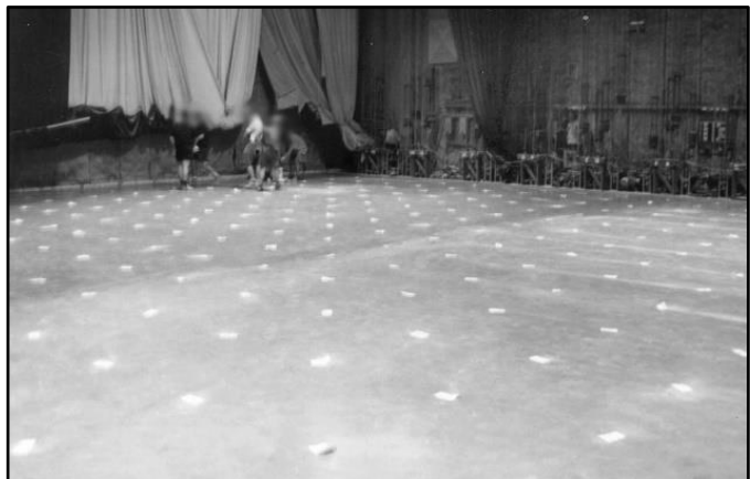
Survey pins positioned on the floor with paper attached for visual identification
