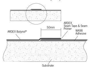
When applying the next sheet, it shall be lapped over the first sheet by 50mm. When the whole area has been covered or as work progresses, the applicator must seal all laps. Overlaps shall be sealed using the ARDEX Seam Tape & ARDEX WPM 299 Seam Primer system.
