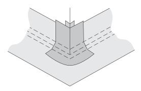
NOTE: Fillets must be used on all internal corners.
