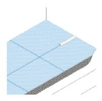
7. Grouting can proceed once the tile bed has hardened sufficiently so that tiles will not be dislodged. Apply ARDEX Grout in accordance with the relevant product data sheet.
