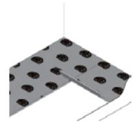
5. Commence tiling using an ARDEX Tile Adhesive. With the trowels flat side, skim a coat of tile adhesive into the fibre glass weave ensuring full coverage before trowelling remaining tile adhesive with the correct notch size (wet on wet application).
