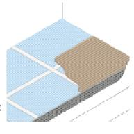
2. Measure and cut ARDEX UD 150 matting to acheive the correct fit, placing mat with seams butted. Ensure the fibreglass weave is facing upwards.
