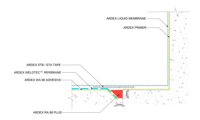
HORIZONTAL REGLET TERMINATION WITH LIQUID MEMBRANE TRANSITION (ARDEX STB TAPE) -OPTION 2
