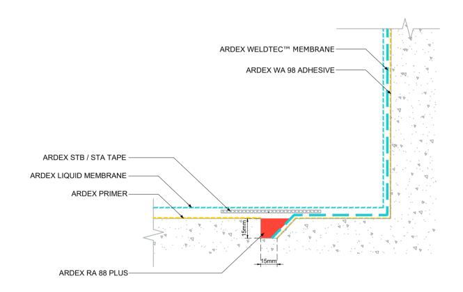
HORIZONTAL REGLET TERMINATION WITH LIQUID MEMBRANE TRANSITION (ARDEX STB TAPE) -OPTION 1
