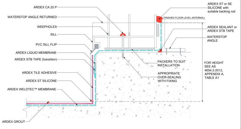
TERMINATION AT EXTERNAL DOOR OPENINGS NO SUB SILL -MODIFIED OPTION 2
