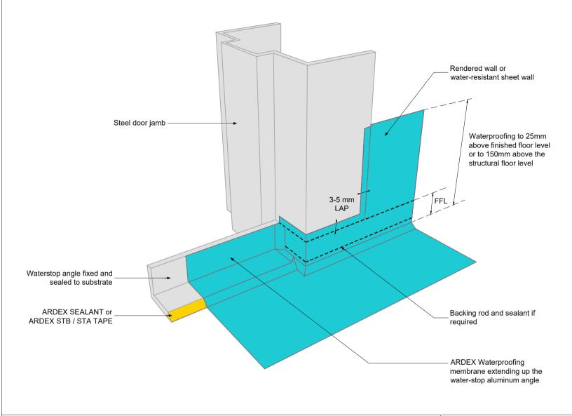
3D - ARDEX WATERPROOFING AT DOOR WITH STEEL FRAME
