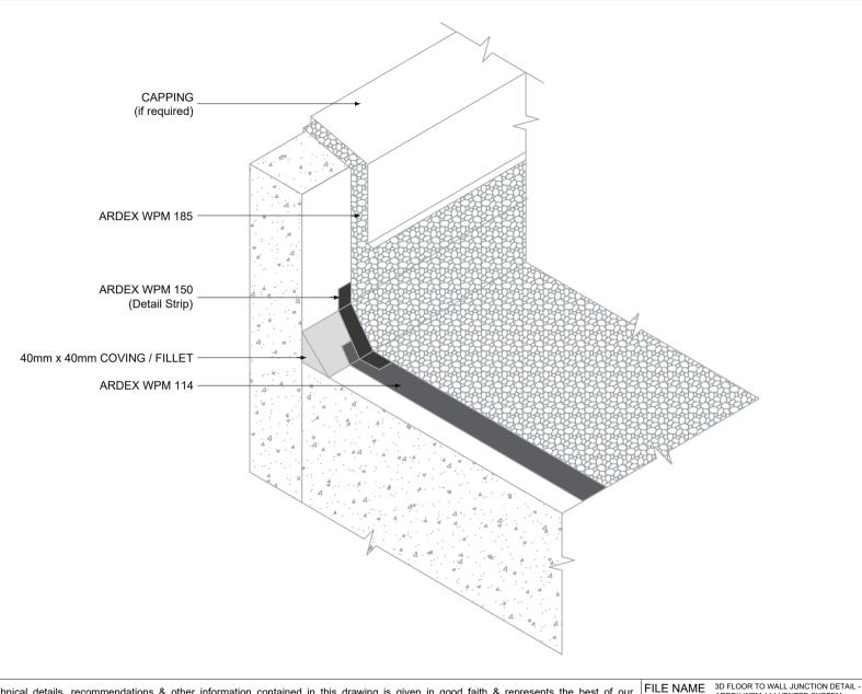
3D FLOOR TO WALL JUNCTION DETAIL - ARDEX WPM 114 VENTED SYSTEM
