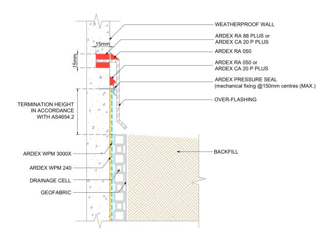
VERTICAL TERMINATION WITH OVERFLASHING & ARDEX PRESSURE SEAL -ARDEX WPM 3000X MEMBRANE
