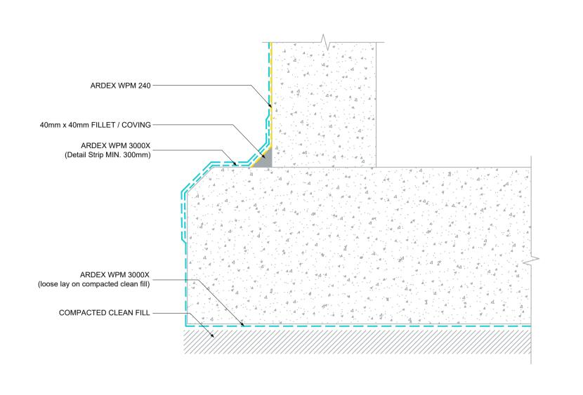
BELOW GROUND FOOTING DETAIL (COMPACTED CLEAN FILL) - ARDEX WPM 3000X
