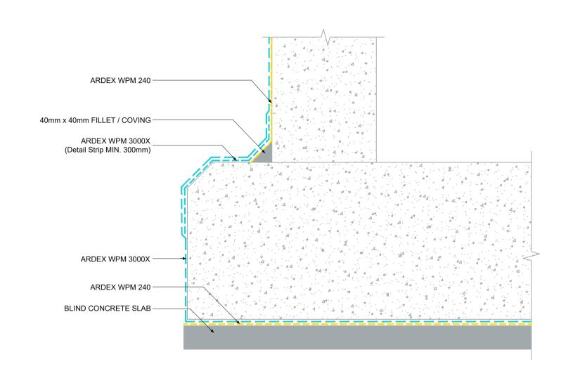
BELOW GROUND FOOTING DETAIL (BLIND CONCRETE SLAB) - ARDEX WPM 3000X
