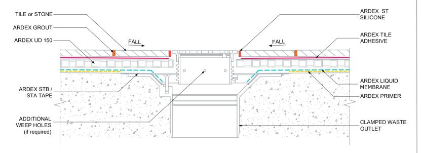
CLAMP DOWN WASTE OUTLET DETAIL -ARDEX UD 150 & ARDEX LIQUID MEMBRANE
