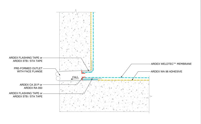
OVERFLOW PIPE DETAIL -ARDEX WELDTEC™ MEMBRANE
