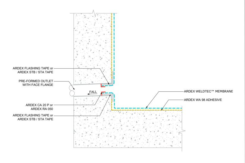
RAISED OVERFLOW PIPE DETAIL - ARDEX WELDTEC™ MEMBRANE
