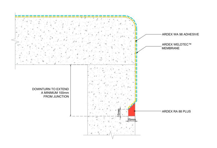
VERTICAL DOWNTURN WITH REGLET TERMINATION - ARDEX WELDTEC™ MEMBRANE
