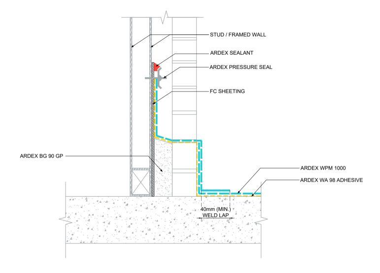
TYPICAL CAVITY FLASHING DETAIL WITH FRAMED WALL & ARDEX PRESSURE SEAL
