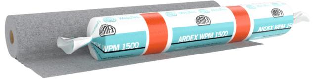
ARDEX WPM 1500 is a pre-applied, fleece-lined, weldable waterproofing membrane for below ground tanking and gas barrier applications. ARDEX WPM 1500 is welded at laps and seams to create a strong, continuous waterproofing membrane. ARDEX WPM 1500 has excellent elongation, flexibility and water migration resistance. The fleece-lined surface allows a high bond strength to concrete.
