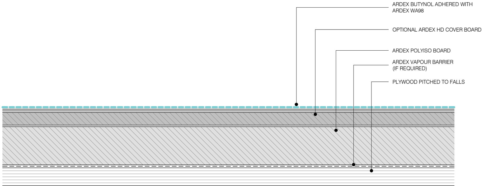
NOTE: FOR FASTENING OR FIXING PATTERN DEPENDENT ON WIND ZONE/R VALUES.
