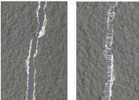
Pictured above: (left) Cracked adhesive without Microtec Technology (right) Cracked adhesive with Microtec Technology.
