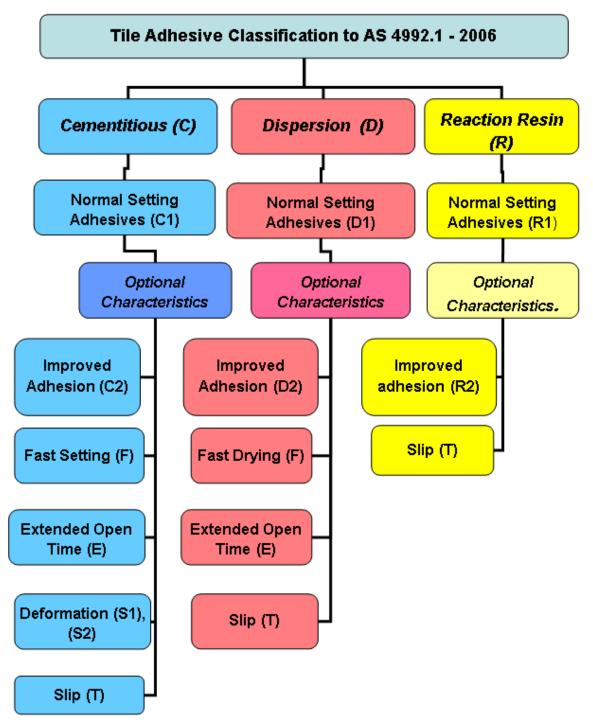
Performance characteristics may be different for each classification, so it is important to correctly identify the type of adhesive being considered. Common descriptive names, such as rubber adhesive or organic adhesive, can confuse, but correct identification ensures the required level of performance.
