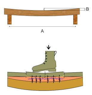
The diagram shows a typical floor or step-tread with the bearer span shown as A and the deflection as B.
