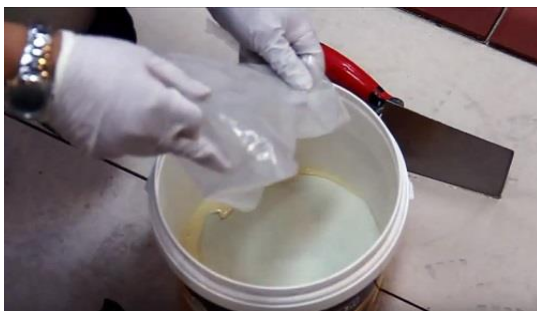
Mixing the combined Parts A+B resins and then adding the filler powder.
