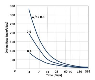
The graph at left shows the effect of increasing the water-cement ratio on the moisture emission rates.
