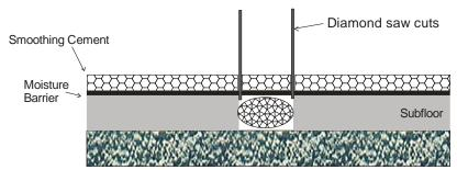
As per step 32, the material from the saw cut has been removed.
