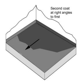
The coats are applied at 90-degree angles to obtain complete coverage.
