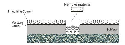
As per step 33, the Moisture Barrier is painted down into the joint. A suitable flexible sealant system is then installed (may include mouldings or metal extrusions
