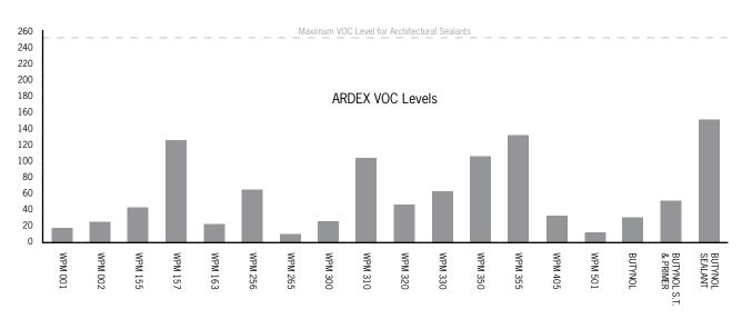
ARDEX waterproofing products have been independently tested by CETEC against the GBCA requirements and fall well under the requirements of 250g/L for IEO-13 Architectural Sealants.
